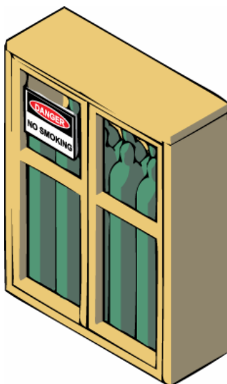
Figure 2-6. Compressed Gas Storage
