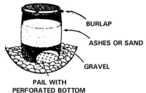
(a) The barrel filter grease trap must be positioned in one of two ways for it to be effective. One is to place trap directly over the soakage pit. The other is to place the barrel on a platform with a trough that leads to the pit.
