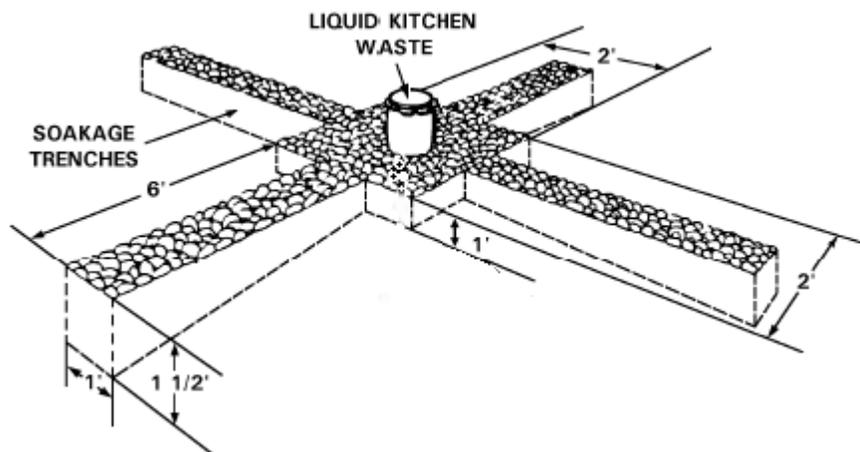
(2) Remember that you will need two soakage trenches for every two hundred persons and each one would require a grease trap. When using two trenches alternate their use to provide each a period of rest. To close the trenches use the same method used for the soakage pit.
