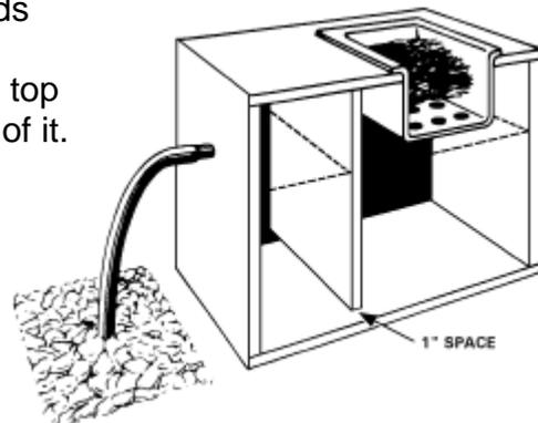
baffle grease trap is properly positioned and the pipe is inserted into the pit, it is ready for use.
