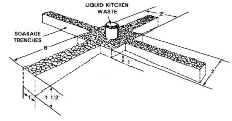
Line the bottom with the same non-porous material as the soakage pit.
