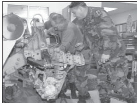
Staff Sgt. Louis Mancuso assists Sgt. Louis Torres in the replacement of a Humvee engine and transmission at Fort Irwin. The Soldiers deployed to the NTC with the 145th Maintenance Company to repair equipment for Operation Iraqi Freedom.
