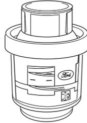
Check the air filter restriction gauge whenever the hood is raised to perform general engine maintenance at least every 7,500 miles (12,000 km). If the vehicle is operated in extremely dusty conditions, check the gauge at least every 500 miles (800 km), or two weeks, whichever comes first.
