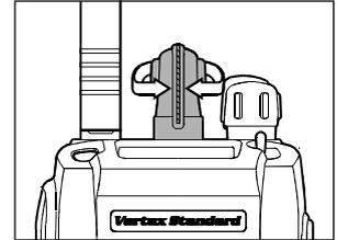
**Note:** Some models are programmed so that the operating channels are selected by the **Soft** key and the memory channel group is selected by the **CH** selector knob. For further details, contact your **VERTEX STANDARD** dealer.
