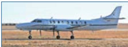
The C-26 Metroliner, a non-standard Army aircraft, is a twin engine turboprop passenger airplane capable of transporting up to 14 personnel for high-priority missions. There are 11 C-26s in the ARNG inventory that fly missions similar to the C-12 when stateside; when deployed overseas, as are two C-26s, these aircraft fly combat support and service support missions.
