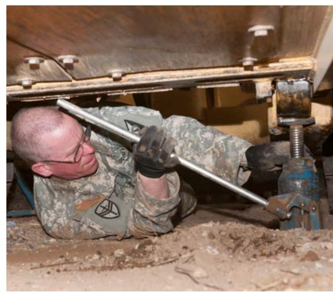
SSG Terry Boulanger, mechanic, 131st Engineer Company, Vermont Army National Guard, lifts a bulldozer to remove the front blade for repairs at Camp Moussa Diom, Bargny, Senegal, February 20, 2015. The 131st Engineer Company was in Senegal to build a humanitarian land mine detection training range with the Senegalese armed forces during their annual training. Senegal is one of Vermont's state partners in the Partnership Program. (Photo by SSG Nathan Rivard.)
