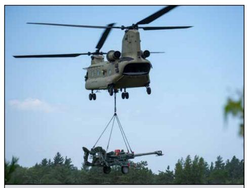
A CH-47 flown by Soldiers assigned to Bravo Company, 3rd Battalion, 126th Aviation carries an M-777A2 howitzer to a firing site during sling load training conducted with the 1st Battalion, 258th Field Artillery at Fort Drum on July 27, 2019.
