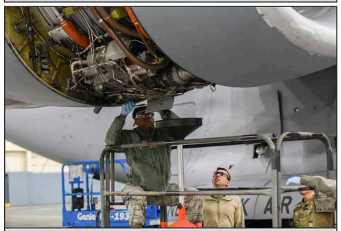
Airman 1st Class Daquiel Duncan and Staff Sgt. Derek Presto of the 105th Airlift Wing Maintenance Squadron, conduct a hard-point inspection during the servicing of a C-17 Globemaster III, March 7, 2020, at the 105th Alrlift Wing, Stewart Air National Guard Base, Newburgh, N.Y.
