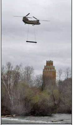
A CH-47 Chinook assigned to Bravo Company, 3rd Battalion, 126th Aviation removes a 3,900-pound steel pontoon (top right photo) from the Niagara River just above the American side of Niagara Falls in Niagara Falls, N.Y., on May 4, 2022.
