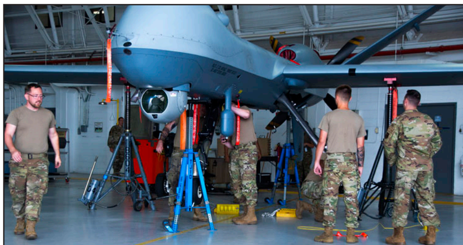
New York Air National Guard Airmen assigned to the 174th Attack Wing's Maintenance Group gather research data to improve weight distribution of the MQ-9 Reaper July 23, 2024 at Hancock Field Air National Guard Base in Syracuse, N.Y.
