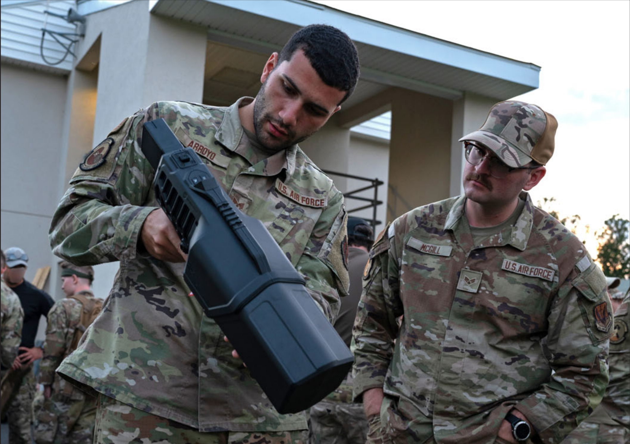
U.S. Air Force Staff Sgt. Anthony Arroyo, left, security forces, 109th Airlift Wing, New York National Guard, and Senior Airman John McGill, right, security forces, 824th Base Defense Squadron, Moody Air Force Base, examine a Dronebuster, a non-kinetic, handheld counter-unmanned aerial system device, during a training event as part of exercise Sage Eagle 25-4 at Fort Anderson-Pinn-Hill, Virginia, Aug. 28, 2025.
