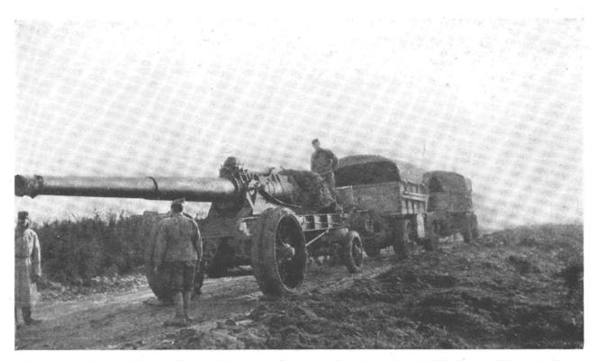
8-inch naval gun (French) used to supplement the fire of 52d Field Artillery Brigade
