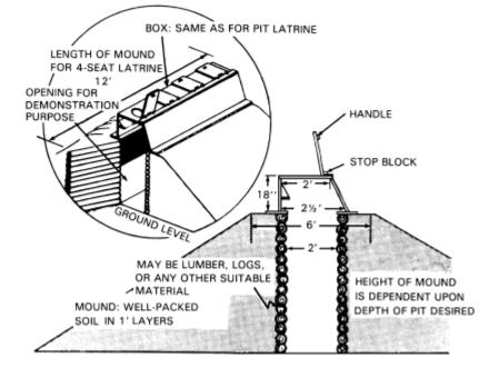
(d) Deep pit latrines. If the unit is going on an extended stay, longer than three days, then deep pit latrines are usually built. This latrine uses a two-seat or four-seat box either issued to, or built by, the unit using. The two-seat box is four feet long, two and one half feet wide at the base, and sixteen inches high. The four-seat box
