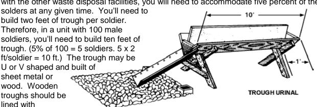
heavy tarpaper. The legs on one end of the trough should be slightly shorter. A pipe is then connected to this end to carry the urine to the urine soakage pit.
