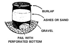
(b) Like all of our field sanitation devices, the barrel filter grease trap requires some maintenance to operate efficiently. Every two days empty and wash the trap. Then refill it with fresh ashes or sand. Wash or replace the burlap strainer daily. Burn or bury the ash or sand to prevent infestations from pest or insects.
