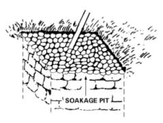
a soakage pit you should first mound it over with one foot of compacted soil. The compacted soil will keep insects and vermin from entering and exiting the pit. Then post a sign on the mound that states the type of pit and the date it was closed.
