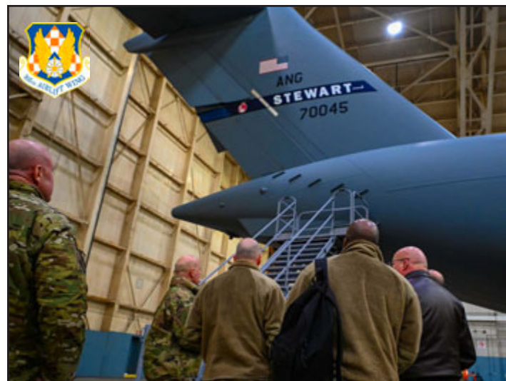
New York Air National Guard and Stewart Air National Guard Base leadership look at a C-17 Globemaster III equipped with Microvanes, at Stewart ANGB, New York, Feb. 2, 2025. Microvanes are 3D printed devices that when installed on the rear of a C-17, reduce both drag and fuel consumption by one percent, saving the Air Force money and enhancing mission capability.
