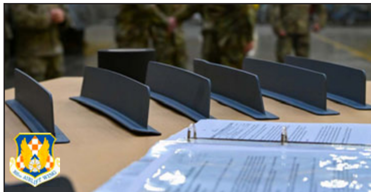
Microvanes sit on a table prior to getting installed on a C-17 Globemaster III at Stewart Air National Guard Base, New York, Feb. 2, 2025. Microvanes are 3D printed devices that when installed on the rear of a C-17, reduce both drag and fuel consumption by one percent, saving the Air Force money and enhancing mission capability.
