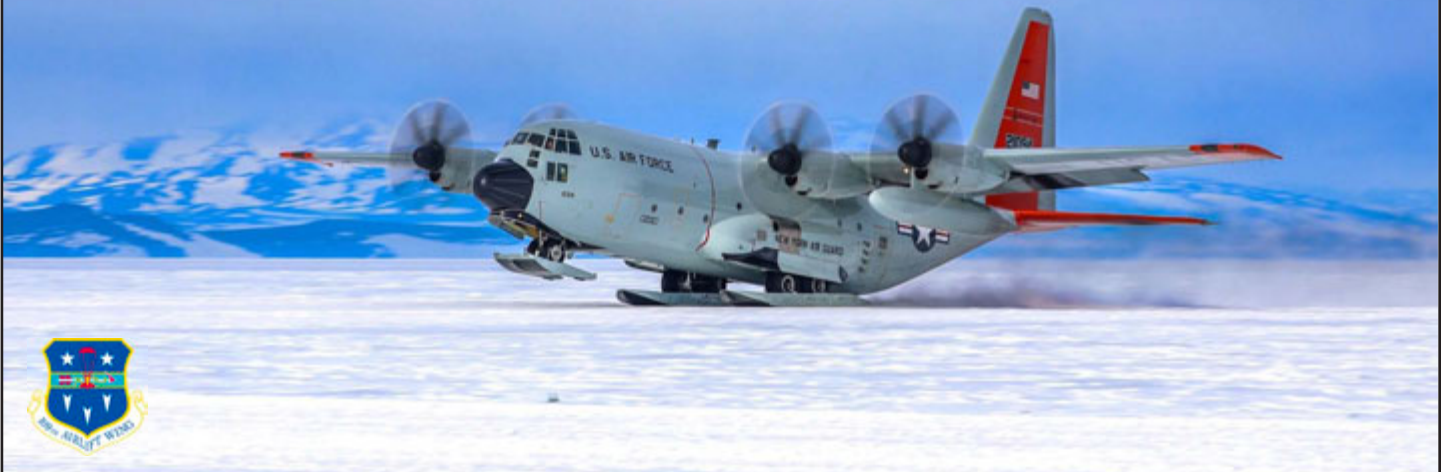
A U.S. Air Force Airman monitors a LC-130 Skibird while it offloads cargo at the South Pole Station, Antarctica. The New York National Guard's 109th Airlift Wing flies the LC-130 in support of Operation Deep Freeze, supporting the National Science Foundation in Antarctica. The LC-130 Skibird is a variant of the C-130 Hercules aircraft, the Skibird is the only heavy airlift in the world equipped with skis to land on snow and ice. (U.S. Air National Guard photo by Tech. Sgt. Gabriel Enders, 109th Airlift Wing.)
