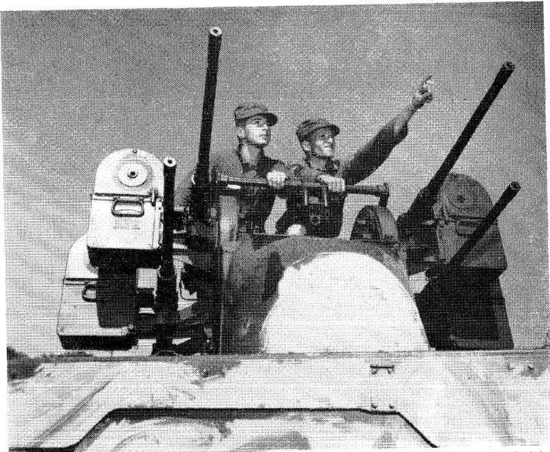
Four electrically operated 50 Cal. Machine Guns manned by men of the 142d AAA AW Bn (SP) sight approaching aircraft at Camp Drum, New York during summer Field Training
