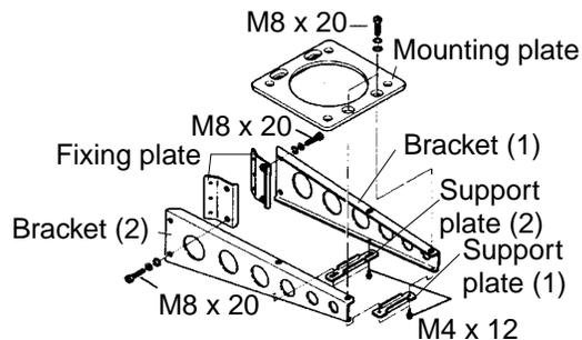
**(A) Assembling the mounting bracket**
