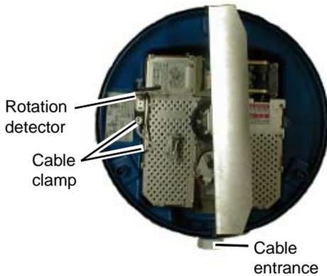
*Antenna unit, cover removed, top view*
