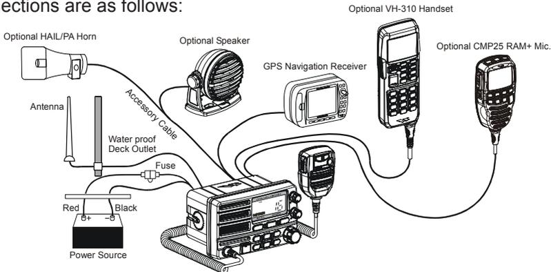
1. Mount the antenna at least 3 feet away from the radio. At the rear of the radio, connect the antenna cable.
