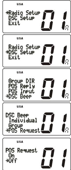
If you wish to return to enabling the ringer tone, just repeat the above procedure, turning the **CHANNEL** selector knob to select “On” in step “6” above.
