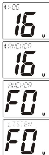
To exit from the FOG HORN mode, press and hold down the **[NAV]** key again.
