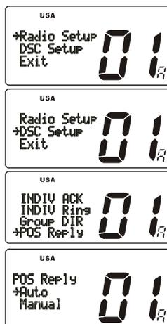
The **GX3000S** has the capability to turn off the Position Request ringer.
