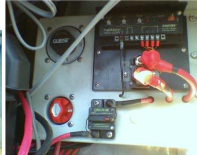
(Battery Isolator – Starboard Side Aft)
