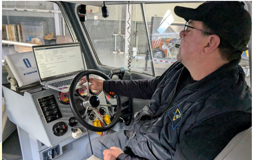
MK1 Keith White conducting analysis of the PB281 starboard engine using Mercury G3 computer diagnostics.
