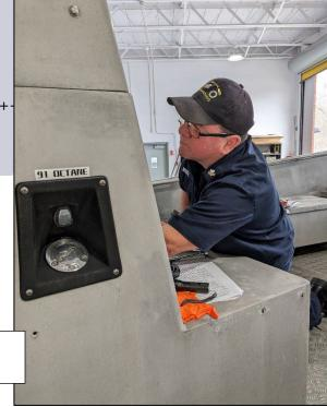
MK2 White traces a ground in the fuel gauge circuit of PB220.
