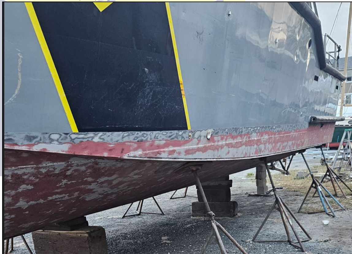
PB 400 bottom after soda-blasting.
