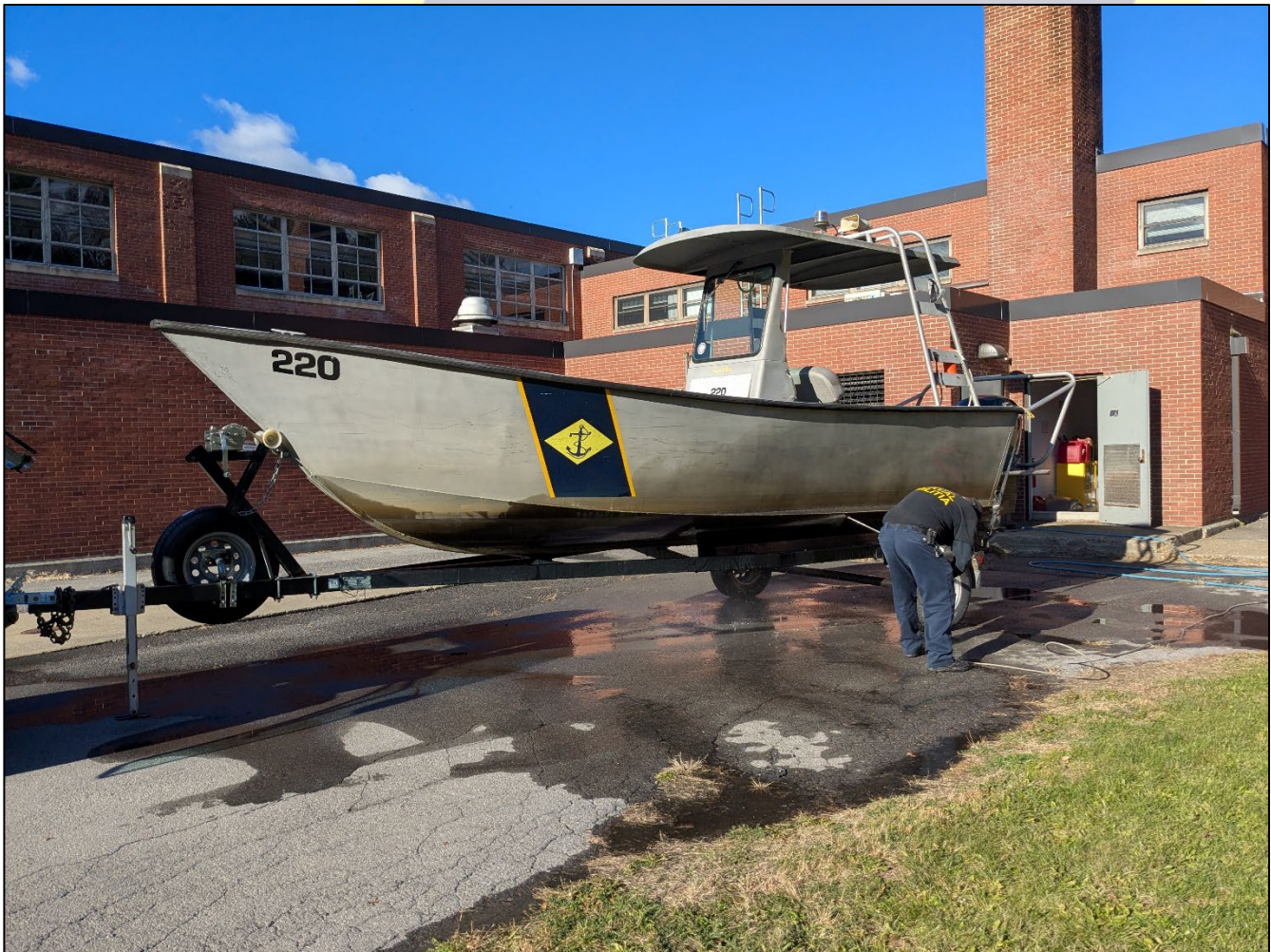
Power-washing hull bottoms
