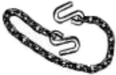
provisions for the connection of **safety chains**, which are required by most states. When connected, safety chains should have some slack to permit sharp turns but should not drag on the road. In addition, they should cross under the trailer tongue to help prevent the tongue from dropping to the road in the event the trailer separates from the tow vehicle.
