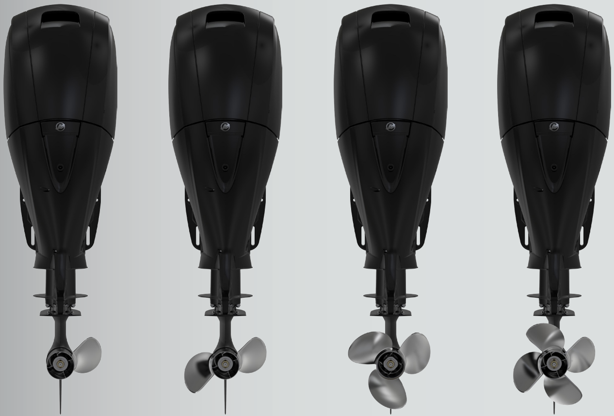
FIGURE 7 VIBRATION LEVEL As blades are added, efficiency and vibration level decrease.
